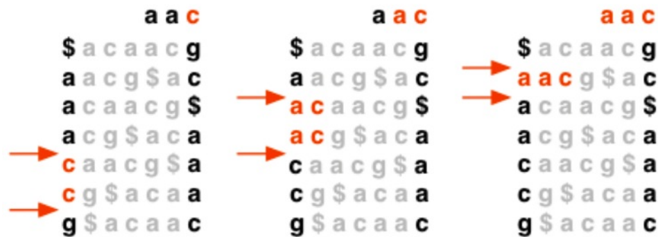
Figure 2.17: Steps to match the substring “aac” in the string “acaacg$” [13].
